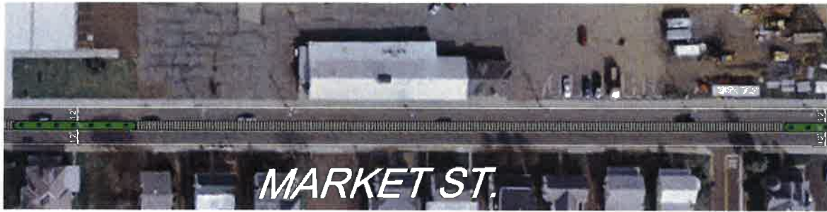
Figure 4 - Center raised landscaped medians and a center flush concrete/stamped asphalt median
