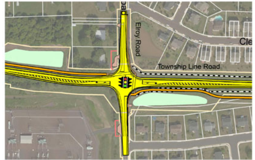
Image from the Pa309connector.com website showing the new shared use path in orange along the proposed PennDOT project.
