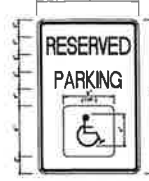
RESERVED PARKING SIGN (R7-3) LEGEND AND BORDER - GREEN (NON-REFLECTIVE) BACKGROUND - WHITE (NON-REFLECTIVE) LETTERS - WHITE (NON-REFLECTIVE) BACKGROUND - BLUE (NON-REFLECTIVE)
